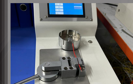
Terminal Pull Test
