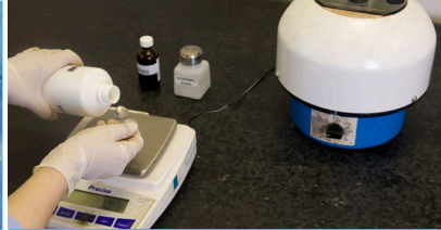
Epoxy Amount Measuring
