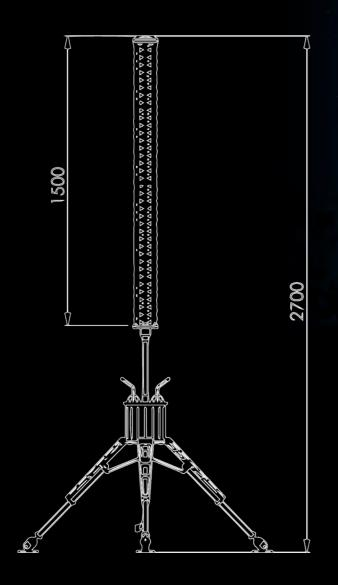
Body Material Lens Angle Power Consumption Source of Light Operating Voltage Color Temperature CRI IP Class Luminous Flux (Im) Aluminum + PC 360° 216W / 120W Mid Power LED 20~28 VDC / 100~277 VAC 2200K~6500K >80 IP65 16800 Im ~ 21150 Im
